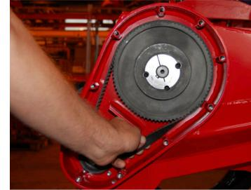
Another way to check the tension is to try to turn the belt 90°. This should be possible but only with a very firm hand.
