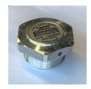
To solve this problem we have tested to use a completely sealed cap instead of the original cap.
