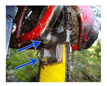
Chain tensioning based on excentric movement.
