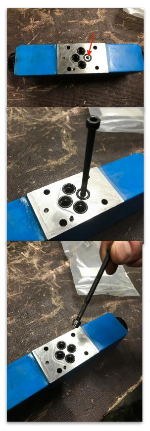
Before changing the electromagnetic valve, please check if it has orifice plugs.
