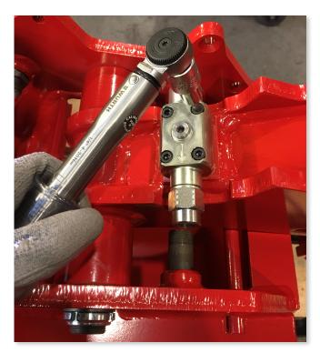
Attach the pump to it's place. Cross tighten the bolts with a torque wrench about 8 Nm.
