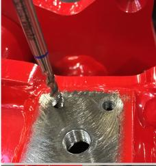
Clean the threads with a M6 thread tap.
