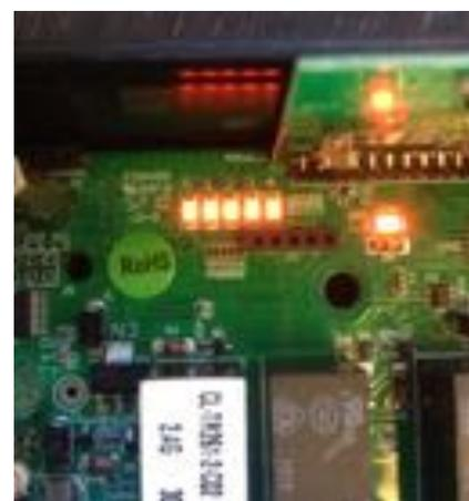
**NOTE! If the “Function” LED on the receiver blinks red, one or more transmitters are paired to the receiver.**
