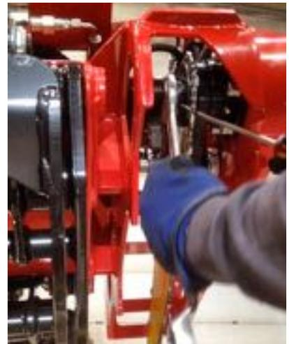
3. The chain releases from the pulley, remove the chain.
