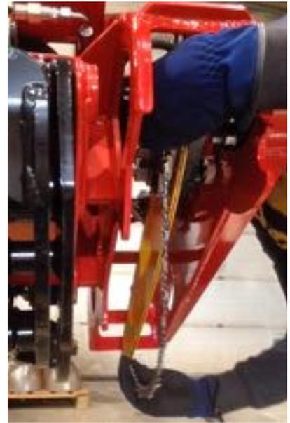
3. Then turn the nut for the pulley downward until the chain is on.
