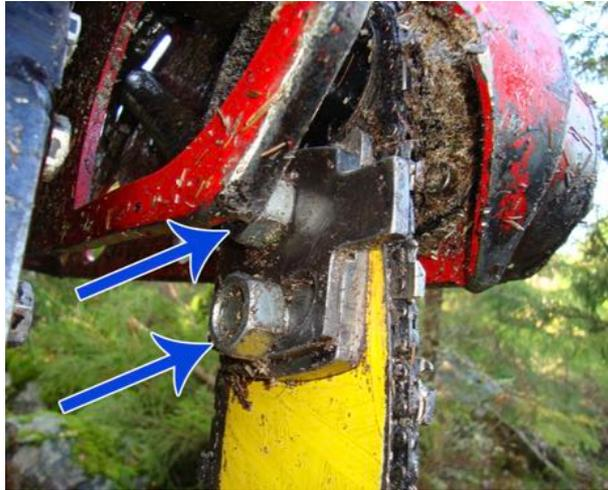
Tension the chain by hand, this should be enough. Alternatively the same wrench which fits the nuts will fit the tensioner also.
