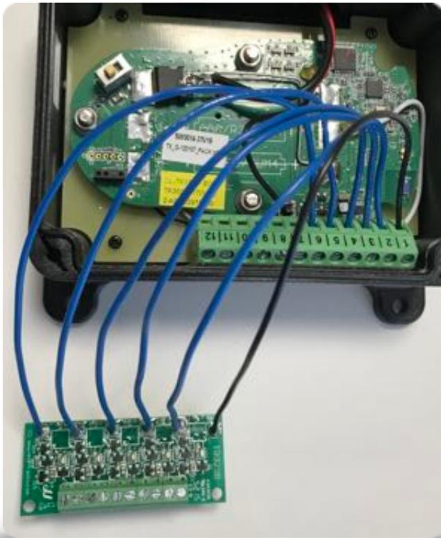
Any input can be assigned to any channel on the transmitter, as long as it's grouped to the same common connector (1 or 7).
