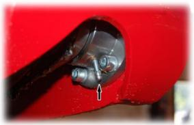
Lubricate the saw bar attachment in 80-100 h intervals.
