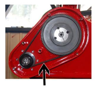
If the grapple saw is used while the drive belt is loose, the belt may be worn out in just a few days.
