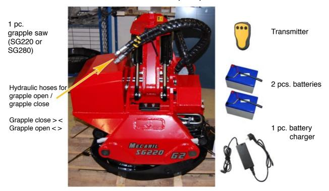
If the grapple saw is ordered with rotator and link, the delivery will also include bolts for installation as well as hydraulic fittings for the grapple hoses to rotator.
