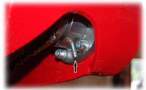
*Lubricate the saw bar attachment in 80-100 h intervals.*
