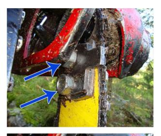
Tension the chain by hand, this should be enough. Alternatively the same wrench which fits the nuts will fit the tensioner also.
